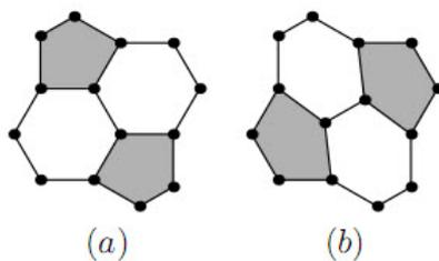
Figure 1: Stone-Wales rearrangement which replaces the patch (a) by the patch (b).
