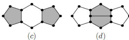
Figure 2: Endo-Kroto C2 insertion which exchanges the patch (c) for the patch (d), and then inserts two new vertices.
