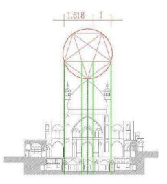
Figure 31: Elevation geometry in the Aghabozorg Mosque.
