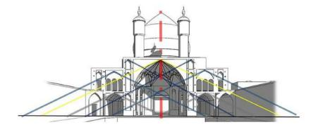
Figure 20: Elevation geometry in the Aghabozorg Mosque.
