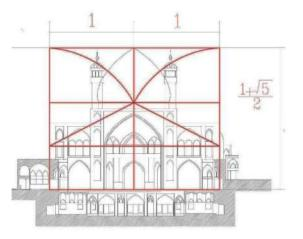
Figure 32: Elevation geometry the Aghabozorg Mosque, composed of two rectangles with a golden ratio of 1.618.
