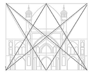
Figure 24: Elevation geometry in the Aghabozorg Mosque.
