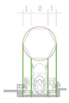
Figure 30: Elevation geometry in the Aghabozorg Mosque.
