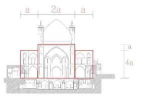
Figure 21: Elevation geometry in the Aghabozorg Mosque.
