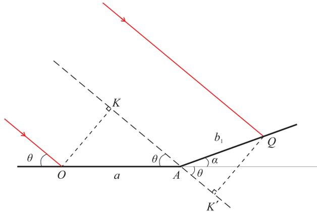
Figure 7: Incident parallel rays that strike the reflector at points  $O$  and  $Q$  such that  $|OA| = a$  and  $|AQ| = b_1$  as in [Theorem 2.2](#), are symmetric with respect to the line passing through  $A$  and parallel to the incident rays.
