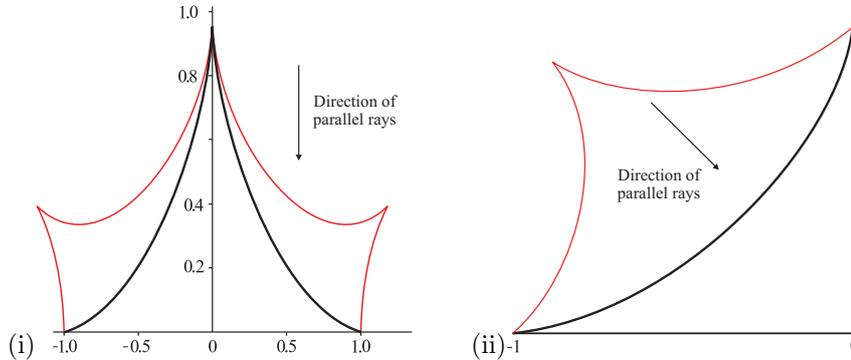
Figure 24: The reflector curve  $\gamma(t) = (\cos^3(t), \sin^3(t))$  (black) and the image curve (red). The incident angle is  $\theta = 90^\circ$  in (i), and  $\theta = 45^\circ$  in (ii).
