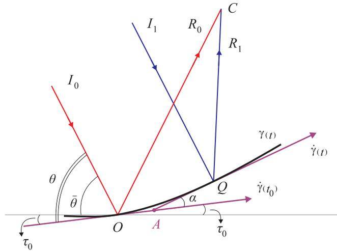
Figure 10: Angles  $\theta$ ,  $\bar{\theta}$ ,  $\tau_0$  and  $\alpha$  are shown for the reflection of two distinct rays which are parallel before incidence to the reflector and have a crossing point  $C$  in front of the parametric curved reflector  $\gamma$ .
