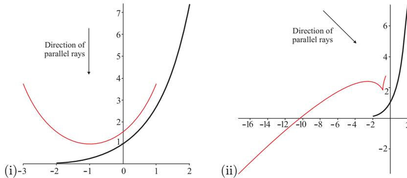
Figure 21: The reflector curve  $\gamma(t) = (t, e^t)$  (black) and the image curve (red). The incident angle is  $\bar{\theta} = 90^\circ$  in (i), and  $\bar{\theta} = 45^\circ$  in (ii).
