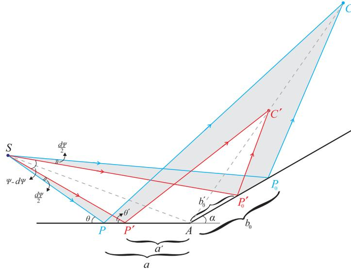
Figure 6: The interference points  $C$  and  $C'$  of the rays which are sent from a source  $S$  to the joint flat walls, are on a line passing through the joint point of the walls.
