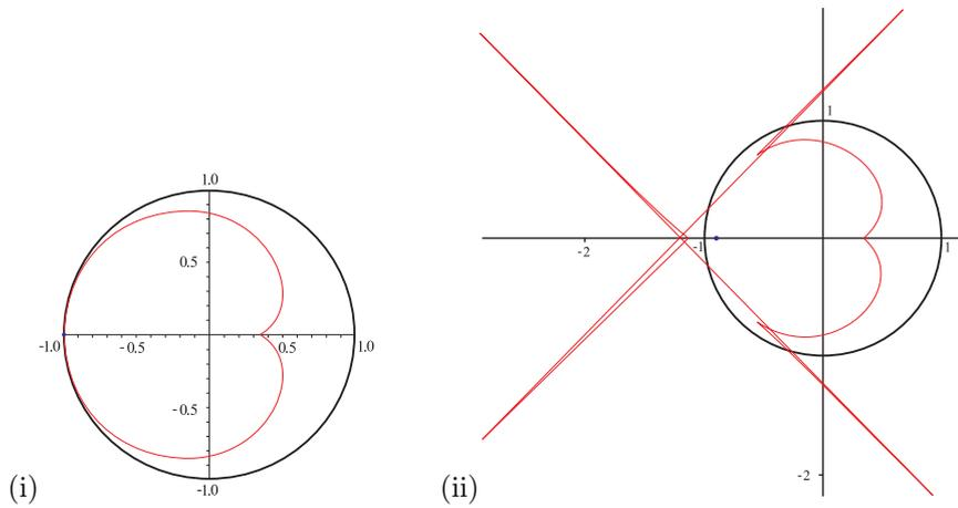
Figure 12: For the circle  $\gamma(t) = (\cos t, \sin t)$  the intersections of reflected rays (red color thin curves) are drawn for  $S = (-1, 0)$  in (i), and  $S = (-0.9, 0)$  in (ii), that in (i) the image curve is a cardioid.
