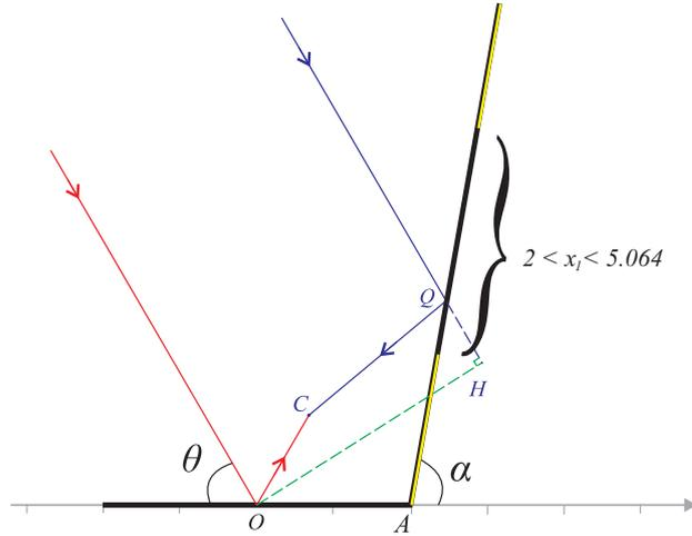
Figure 4: When the distance  $x_1 = |AQ|$  is in the interval defined by [Theorem 2.2](#), it is possible that  $\overline{HQ} < 0$  and the interference point  $C$  is in front of the reflector (see [Example 2.3\(b\)](#) for details).
