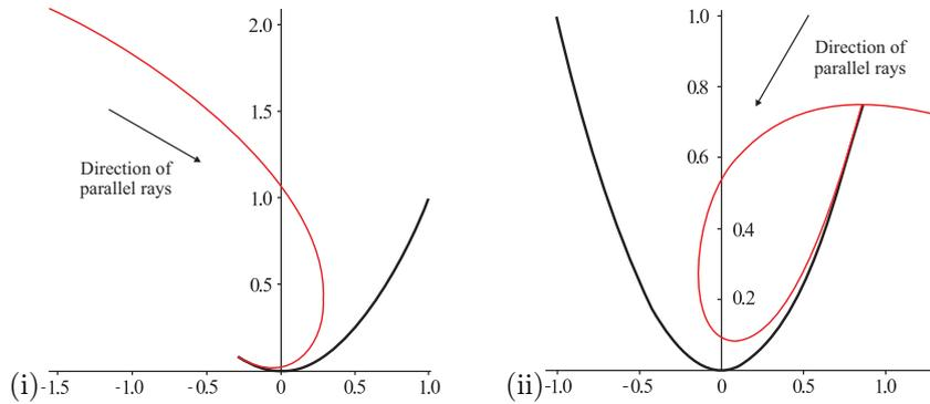
Figure 19: The reflector curve  $\gamma(t) = (t, t^2)$  (black) and the image curve (red). The incident angle is  $\bar{\theta} = 30^\circ$  in (i),  $\bar{\theta} = 120^\circ$  in (ii).
