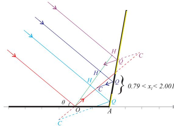
Figure 3: For a fixed ray that is reflected at point  $O$  on the first wall of the reflector, the crossing point  $C$  may be in front of or behind the reflector, depending on the place of point  $Q$  on the second wall. If the distance  $x_1 = |AQ|$  is in the interval defined by Theorem 2.2, the crossing point  $C$  may have the role of the interference point and will be in front of the reflector.
