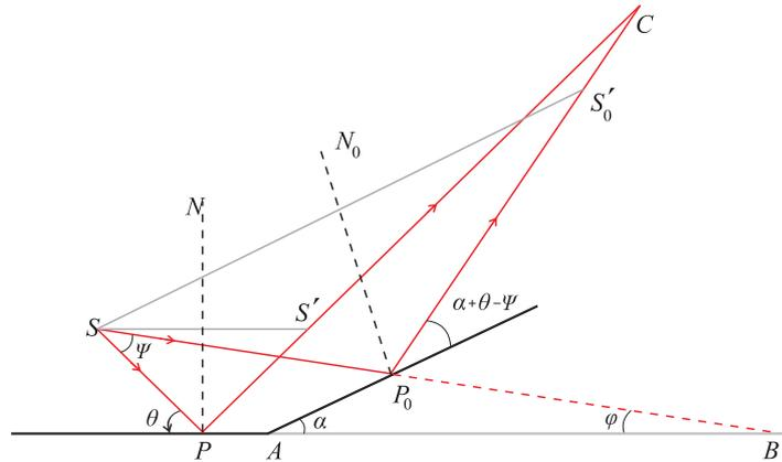
Figure 1: The reflection of two distinct rays which are sent from a source  $S$  and have a crossing point  $C$  in front of the reflector that consists of two flat reflectors. The angle  $\alpha$  between these reflectors, which is shown at the joint point  $A$ , is the angle between two normals  $N$  and  $N_0$ . The points  $S'$  and  $S'_0$  through which pass reflected rays are symmetrical points to  $S$  with respect to normals  $N$  and  $N_0$ , respectively.
