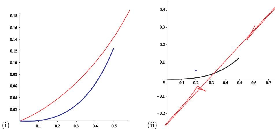
Figure 11: The reflector curve is  $\gamma(t) = (t, t^3)$ . The (red color) thin curves of intersections of reflected rays are drawn for the source point  $S = (0, 0)$  in (i), and  $S = (0.2, 0.05)$  in (ii).
