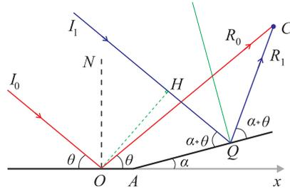
Figure 2: The reflection of two distinct parallel rays which have a crossing point  $C$  in front of the reflector consists of two flat reflectors.
