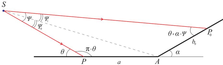
Figure 5: Incident rays  $SP$  and  $SP_0$ , which strike the reflector at points  $P$  and  $P_0$  such that  $|PA| = a$  and  $|AP_0| = b_0$  as in [Theorem 2.1](#), are symmetric with respect to  $\overleftrightarrow{SA}$ .
