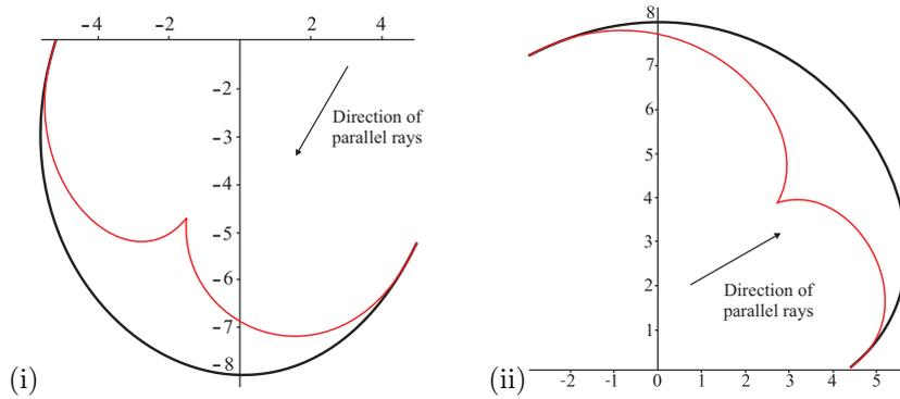
Figure 22: The reflector curve  $\gamma(t) = (6 \cos t - 2 \cos(3t), 6 \sin t - 2 \sin(3t))$  (black) and the image curve (red). The incident angle is  $\bar{\theta} = 120^\circ$  in (i), and  $\bar{\theta} = -30^\circ$  in (ii).
