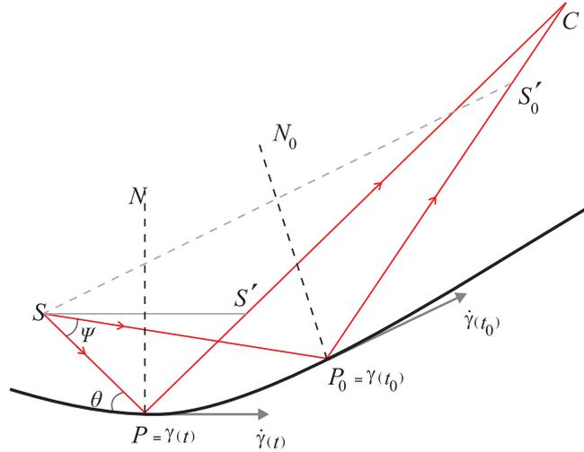
Figure 9: The reflection of two distinct rays which are sent from a source  $S$  and have a crossing point  $C$  in front of the parametric curved reflector  $\gamma$ .
