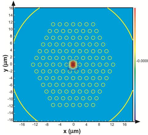
Figure 5: The field distribution of the first-order mode for the first proposed IGPCF at  $\lambda=1.55\mu\text{m}$ .
