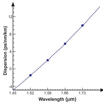
Figure 7: The chromatic dispersion curve of the second proposed IGPCF as a function of wavelength.
