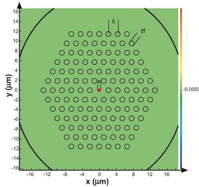
Figure 1: The cross section of the first proposed IGPCF with  $d_1=780$  nm,  $\Lambda=2300$  nm, and  $d_c=400$  nm.
