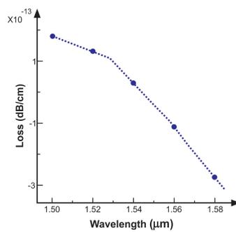
Figure 8: The confinement loss curve of the secondary proposed IGPCF with respect to the wavelength.
