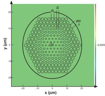
Figure 6: The cross section of the second proposed IGPCF with  $d_1=780$  nm,  $d_2=1300$  nm,  $d_3=1800$  nm, and  $\Lambda=2300$  nm.
