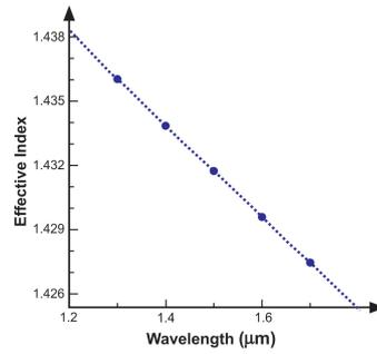
Figure 9: The effective index curve of the second proposed IGPCF with respect to the wavelength.
