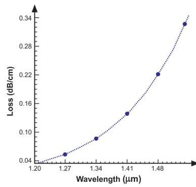
Figure 3: The confinement loss curve of the first proposed IGPCF as a function of wavelength.
