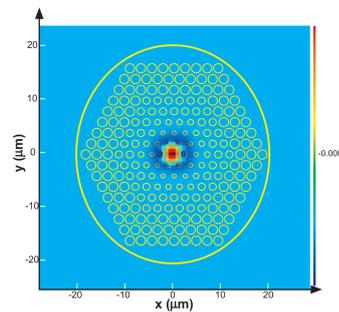
Figure 10: The field distribution of the first-order mode for the second proposed IG-PCF at  $\lambda=1.55\mu\text{m}$ .
