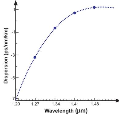
Figure 2: The chromatic dispersion curve of the first proposed IGPCF as a function of wavelength.
