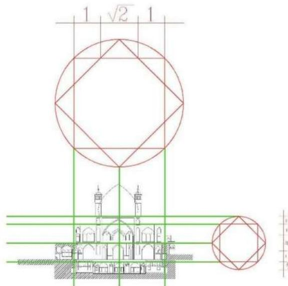
Figure 25: Elevation geometry in the Aghabozorg Mosque.
