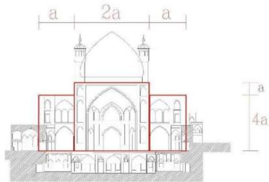
Figure 21: Elevation geometry in the Aghabozorg Mosque.
