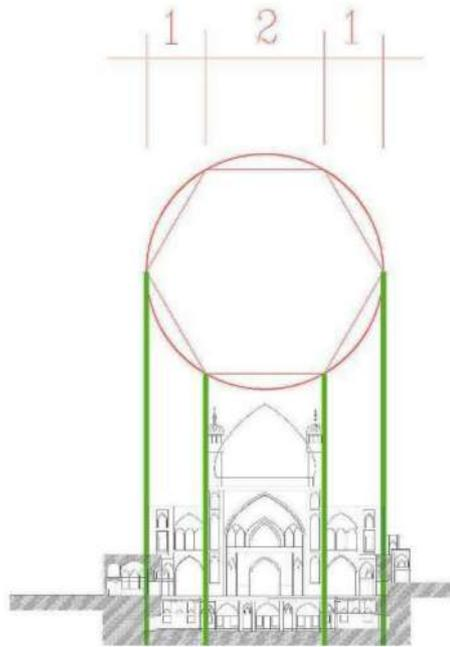
Figure 30: Elevation geometry in the Aghabozorg Mosque.
