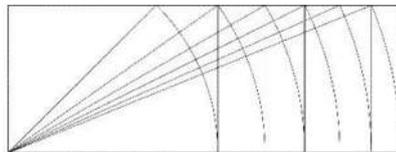
Figure 13: Drawing the rectangle radical 2 and extending it.
