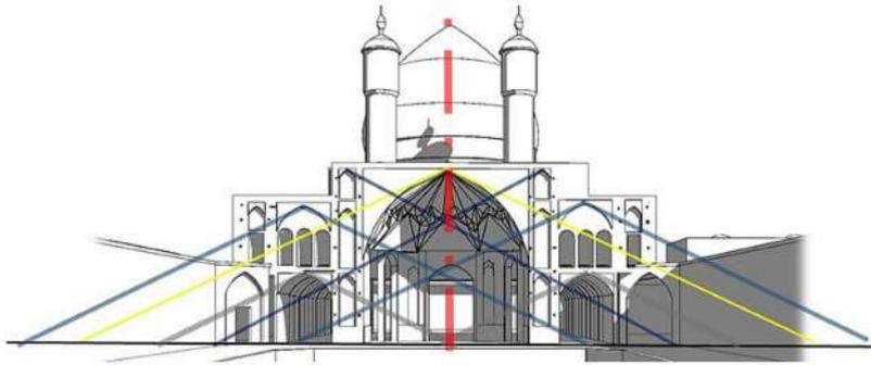
Figure 20: Elevation geometry in the Aghabozorg Mosque.
