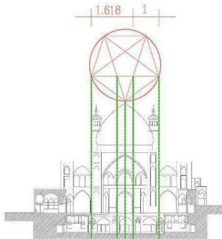
Figure 31: Elevation geometry in the Aghabozorg Mosque.
