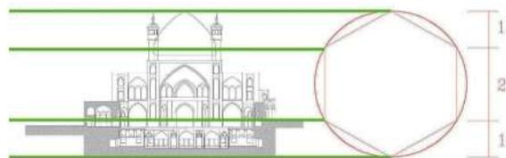
Figure 29: Elevation geometry in the Aghabozorg Mosque.
