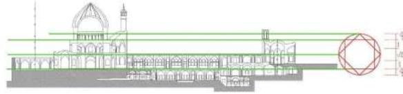
Figure 26: Elevation geometry in the Aghabozorg Mosque.
